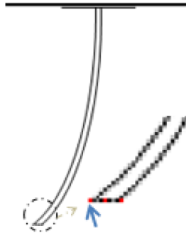
Figure 4.9 Measuring point – end edge.
